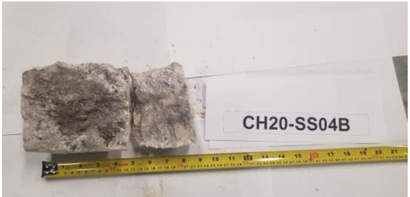
Granular Structure Below Pavement: Gravel fill – poorly graded, medium grained, damp to moist, compact (inferred), light brown
