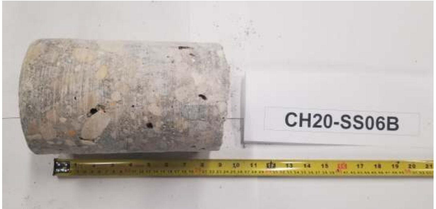
Granular Structure Below Pavement: Gravel fill – sandy, poorly graded, fine grained, damp to moist, compact (inferred), light brown
